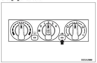
Normally use the "outside" position to keep the windshield and side windows clear and, also to quickly remove fog or frost from the windshield.
